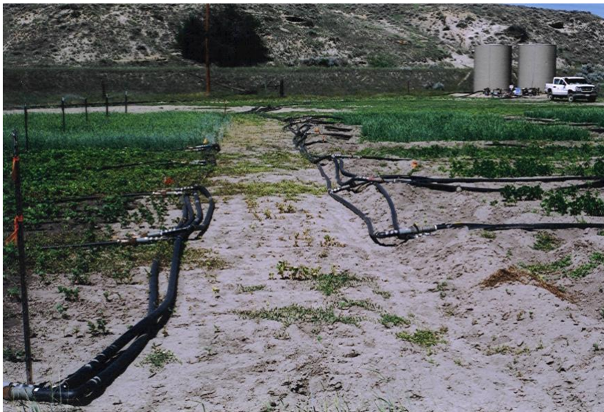
Figure 3. Irrigation system overview, with the flood treatment on the right and sprinkler treatment on the left. Tanks in the upper right of this photo hold Tongue River water (right tank) and CBNG produced water (left tank).
